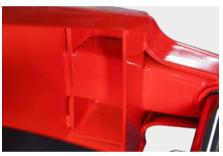
Extra reinforcement rod on top of the chassis.
