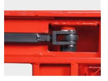
Adjustable push rod: Adjustable push rod design, after 1-2 years use, due to wrong load center, there might be situation with 2 forks not in the same even level, the customer can adjust the forks to even level with the adjustable push rod.
